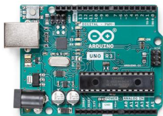
Gambar 1. Arduino Uno (Sumber : https://search.arduino.cc/ )
